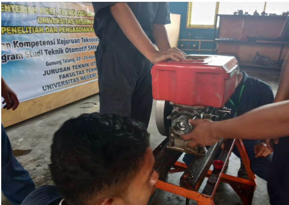
Gambar 22. Praktikum memasang piston engine diesel
