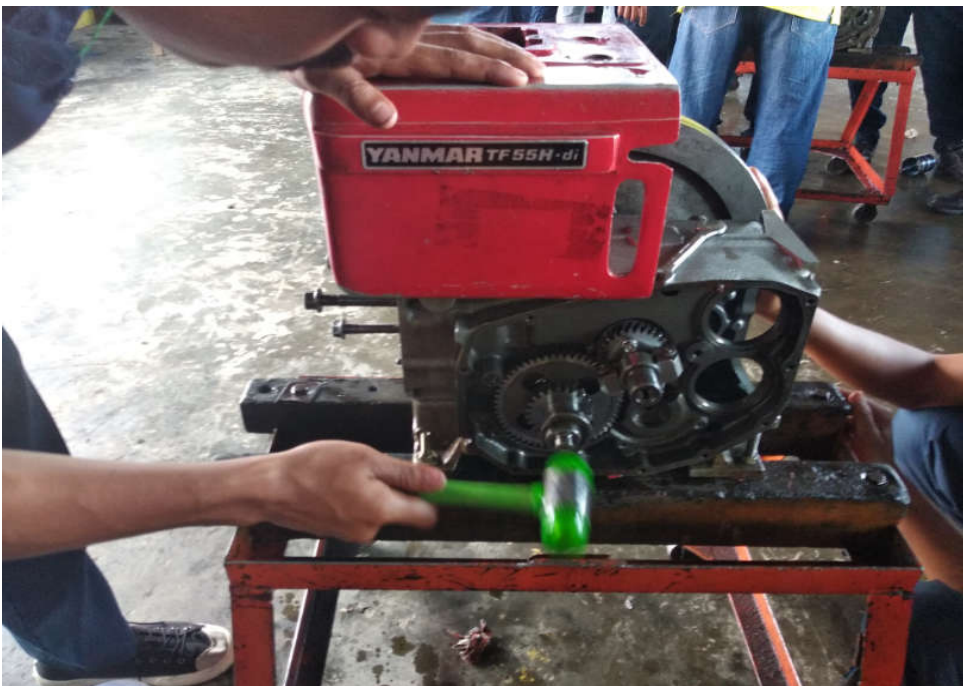
Gambar 24. Praktikum memasang poros nok (cam shaft) engine diesel
